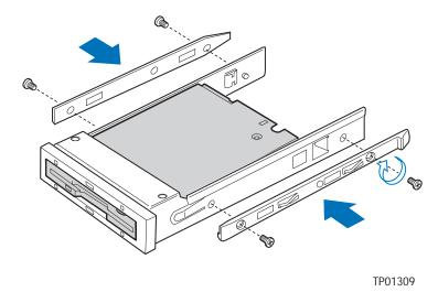
Figure 27. Install the Rails onto the Floppy Drive Conversion Kit Carrier
